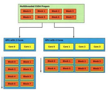
Fig.2. More multiprocessors execute in less time same amount of blocks
